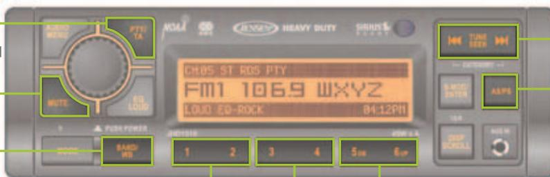
**TUNE:** Press > to tune UP in frequency. Press < to tune DOWN in frequency. Press and hold to fast search.
