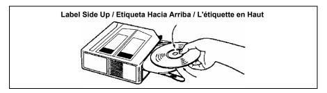
Push the tray back into the magazine. Load discs into the remaining 9 trays in a similar manner.
